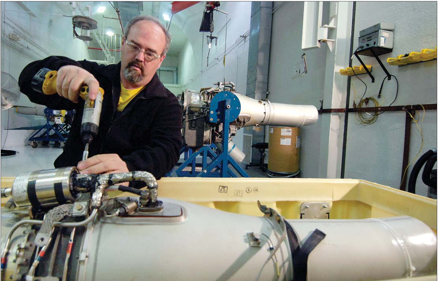
Don Brown removes a start cartridge and oxygen bottle from an F107 cruise missile engine, disarming the engine before it will go for an overhaul. The 550th Commodities Maintenance Squadron Cruise Missile Engine Shop is unique to the Air Force. [Photo courtesy of U.S. Air Force-Margo Wright]
